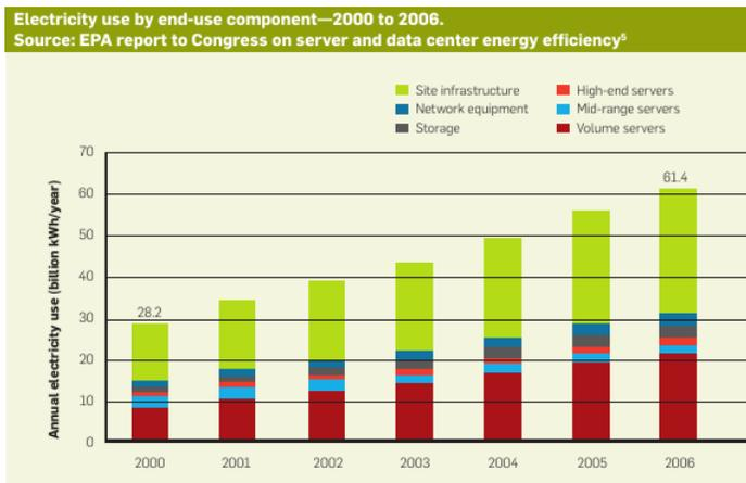
Fig. 1. Graph:Electricity use by end-use component-2000 to 2006. Source [1]
